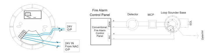
Connect the sounder base to the NAC terminal of a Fire Alarm Control Panel, according to the polarity. The wiring terminal accepts solid or stranded cables up to mm<sup>2</sup>.
