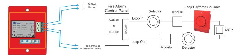
Connect the Loop Positive & Negative wires to SLC IN Terminal, observing the polarity. The wiring Terminal accepts solid or stranded cables up to 2.5 mm<sup>2</sup>.
