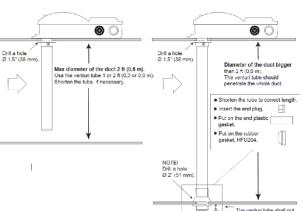
The venturi tube shall not protrude more than 1" (30 mm) through the duct wall.
